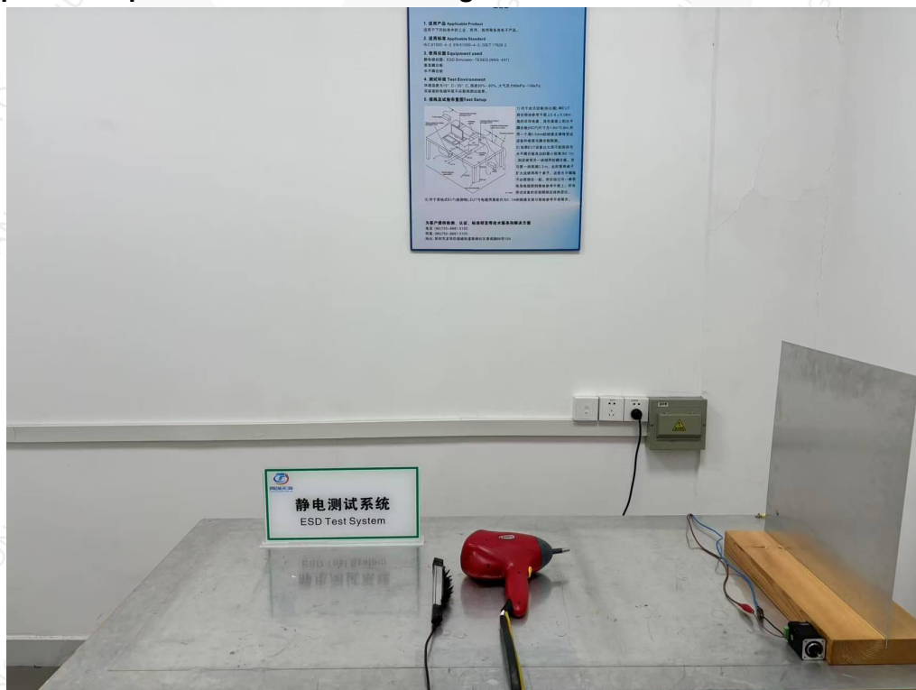
Photograph 2 :Setup for Electrostatic Discharge
